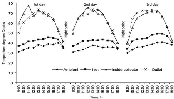
Figure 2. Air temperatures of ambient, at inlet of solar collector, inside solar collector and at outlet of solar collector during the three days of the drying process
